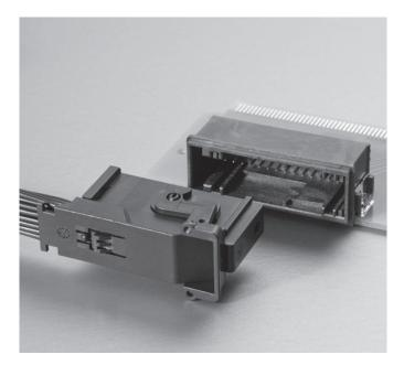
2.54mm pitch, 0.64 unsealed surface mounting type connector with Auto Coplanarity Technology. This technology achieves stable mounting to PCB during re-flow process.
