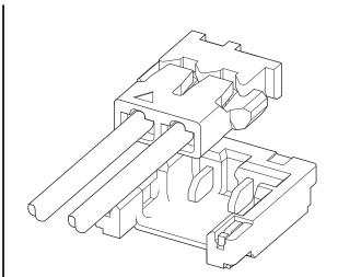
This connector is stacking height 1.2 mm and 1.2 mm pitch.
