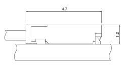
Note: 1. Tolerance for the PCB pattern pitch shall be  $\pm$  0.05 and shall not accumulate. The above dimensions are reference values. Please contact JST for details.
