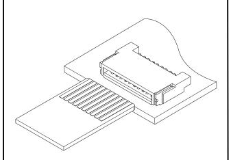
This is a 0.4 mm pitch, compact Non-ZIF type connector with a mounting height of 1.0 mm and a depth of 3.0 mm.
