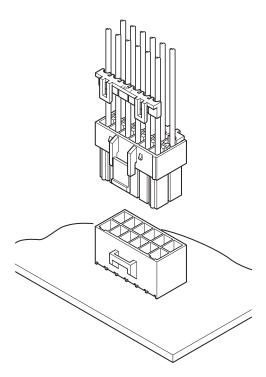
This is a multipurpose product that can also be used for wire-to-board and wire-to-wire connections. A contact with a free spring structure that reduces the stress at the contact part and has excellent creep deformation property and reliability is adopted. In addition, safety design prevents reverse insertion with the boss.
