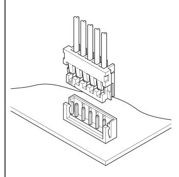
This thin type 2.5 mm pitch connector is an IDC style for PC boards. It is developed by integrating the technologies of crimp style connectors such as EH and PH, and IDC style connectors such as NR, DR, and DB. The In-line method that the wire extraction direction is perpendicular to the board provides high-density wiring.
