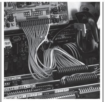
This 2.5 mm pitch insulation displacement connector is another version of the NR connector for printed circuit boards. The NRD connector allows daisy chaining and is very useful in simplifying connection systems in electronic equipment.
