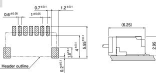
Note: 1. The above figure is the figure viewed from the connector mounting side. 2. Tolerances are non-cumulative:  $\pm$  0.05 mm for all centers.
