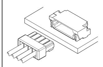
This SUH connector is developed for crimping type SUR connector that has been designed for 0.8 mm pitch wire-to-board insulation displacement connector. This connector adopted the first crimping method in a minimum 0.8 mm pitch of the wire-toboard type connector. Housing lance method provides the good workability and a constriction contact method provides the excellent contact reliability.
