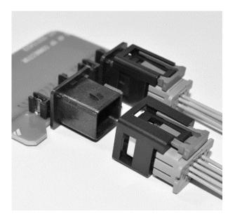
Developed in pursuit of miniaturization and water-proof as surface mounting type connector for automotive. To realize miniaturization and high reliability with the 0.50 terminal and CPA design.
