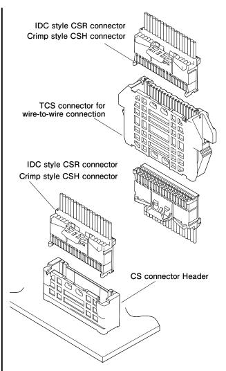
This is a 1.0 mm pitch insulation displacement connector with the secure lock mechanism to prevent coming off the connector and incomplete mating. 1.8 A in rated current was realized by using AWG #27.
