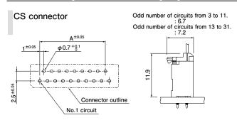
Note: 1. The above figure is the figure viewed from the connector mounting side.
