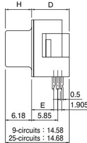
H: Height of the lock screw block (for Types A, B & J)
