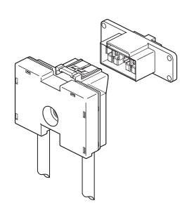
This is a 2-circuit wire-to-wire connector with a 90 A maximum current rating. The connector housing comes pre-loaded with contacts. The wires are terminated by ring tongue terminals which are mounted to the connector by screw. The ring tongue terminals can be replaced by busbars.
