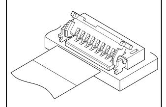
This is a space-saving FPC connector with a low profile of 0.9 mm in mounting height and a depth of 3.1 mm.
