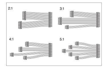
The adoption of the batch termination at branch side and the stitching termination at converged side as the method of insulation displacement connection realizes the template-less (unnecessary template).
