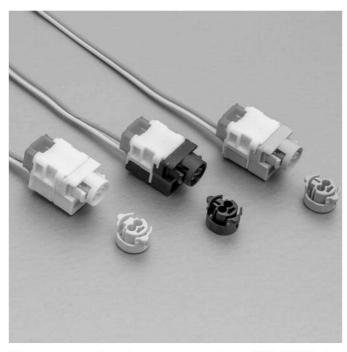
This connector for air-bag, conforming to ISO 19072-4 standard configuration, has intelligent CPA, which allows locking the connector, incomplete mating detection and release of short-circuit in the same time.
