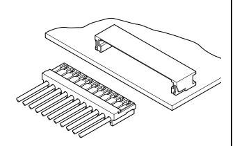
This connector is for wire-to-board connection with 1.0 mm pitch insulation displacement connection, which achieved miniaturization with mounting height 2.0 mm and depth 4.5 mm.
