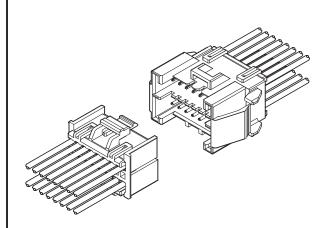
This is a 2.5 mm pitch, dual-row wire-to-wire connector that comes with glow-wire compliant housing material and allows the use of retainers, even on large circuits.
